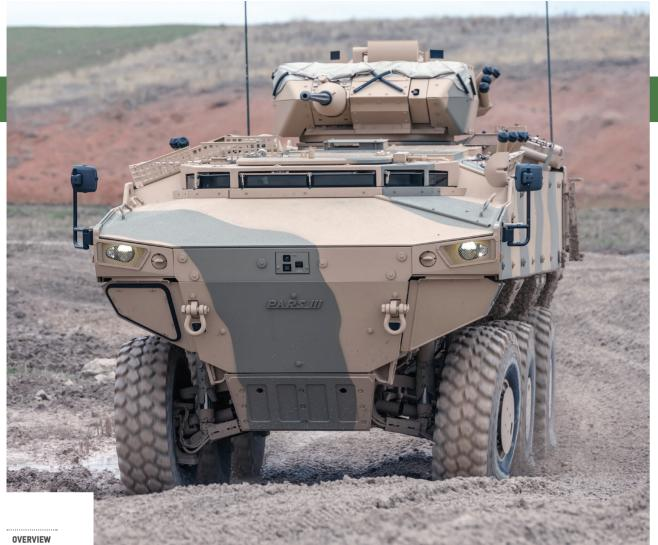
The PARS III 6x6 has been developed with a special emphasis on mobility, protection, payload, and growth potential. It is equipped with cutting edge armoured vehicle technologies to obtain performances and durability answering modern armies' operational requirements.
