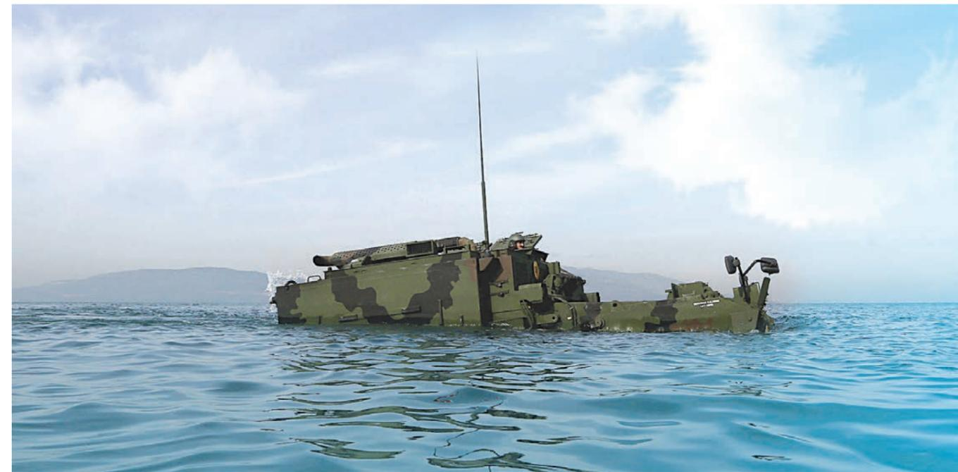
One of the most important and unique features of the AACE is its amphibious capability. It can be operated with a crew of 2. In addition, the AACE is fitted with modern electronic systems such as day and night cameras, multi-function LCD monitor and air-conditioning system.
