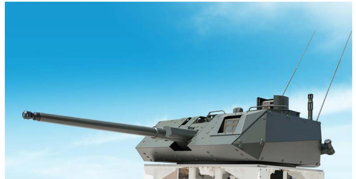
**The TEBER-30 Two-Man Turret, is a medium caliber turret that can be fitted to wheeled and tracked armoured vehicles and is offered in two configurations. In the conventional two-man configuration, the commander and the gunner are positioned in the turret basket.**
