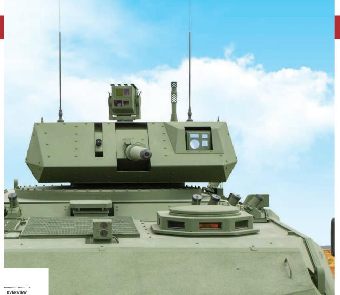
The TEBER-30/35 RCT is a remote controlled turret designed to be installed on wheeled and tracked armoured vehicles and equipped with a medium calibre automatic cannon, an advanced target detection and a fire control system. Unlike conventional turrets, remote controlled turrets do not have any basket structure and thus the extra available interior space provides a significant advantage to the user.
