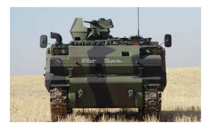
The ACV-19 offers more volume under armour and more payload capacity than the ACV-15. Consequently, the ACV-19 chassis can support heavier payloads such as larger turrets without compromising the mobility offered by the ACV-15. Additionally, the 90% spare part commonality among ACV-19s and ACV-15s makes maintenance more convenient for users of both variants.
