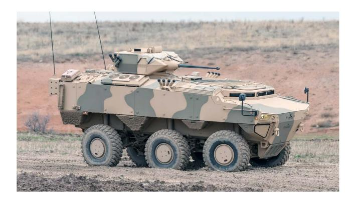
The hull form, underbelly structure, base plates and specially developed mineresistant seats are designed to protect personnel against high-level mine threats. The PARS III 6x6 vehicle runs ahead of its competitors by offering ballistic and mine protections levels similar to MRAP vehicles while maintaining combat and mobility characteristics of modern armoured combat vehicles.
