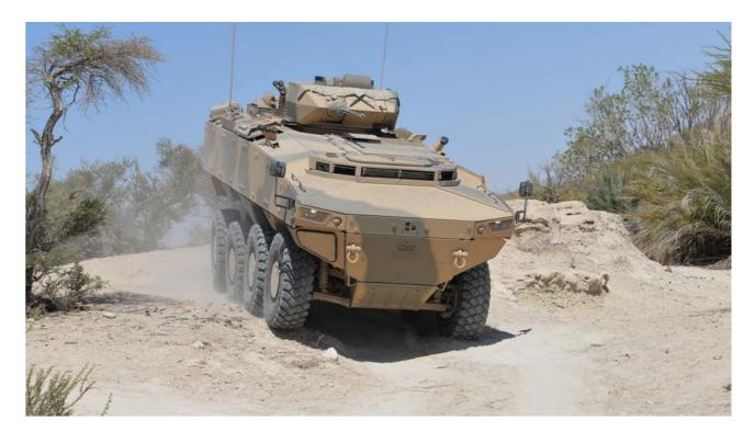
Thanks to the modular design of the PARS III 8x8 hull and to that of its armour package, the vehicle protection level, both against ballistic and mine threats, can be tailored to customers' requests,
