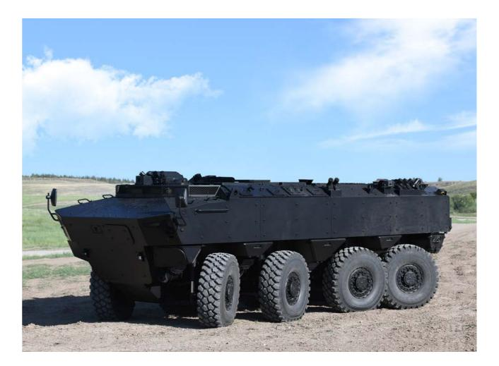
The two-man driver's front cabin of the PARS IV 8x8, allows to operate day and night in all terrain and weather conditions, and provides more than 180° of visibility and a high level of driving safety under armour. Panoramic periscopes at the front of the vehicle, as well as driving and thermal cameras at the front and rear, provide high situational awareness to the driver and commander. This allows performing all kinds of tasks safely under armour protection, without opening the driver's hatch.
