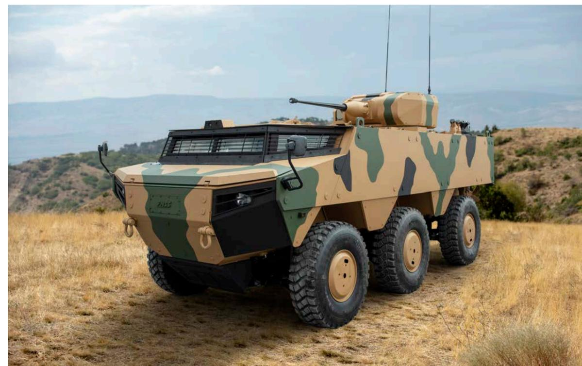
The PARS SCOUT has a range of over 700 km, and it has under-armour protected fuel tanks. The vehicle is fitted with run-flat tires and with a self-recovery winch.
