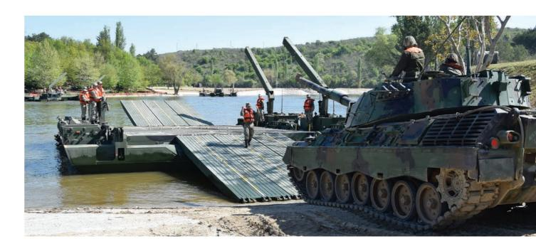
The all-wheel-steering feature minimizes the vehicle's turning radius. The vertical obstacle and trench crossing capabilities are also superior due to the shorter distance between axles in the 8x8 concept. Moreover, the 8x8 configuration gives a maximum axle load of around 9 tons, the significantly low ground pressure providing longer wheel life due to less wear. The OTTER can cope with 60% gradient and 30% side slopes.
