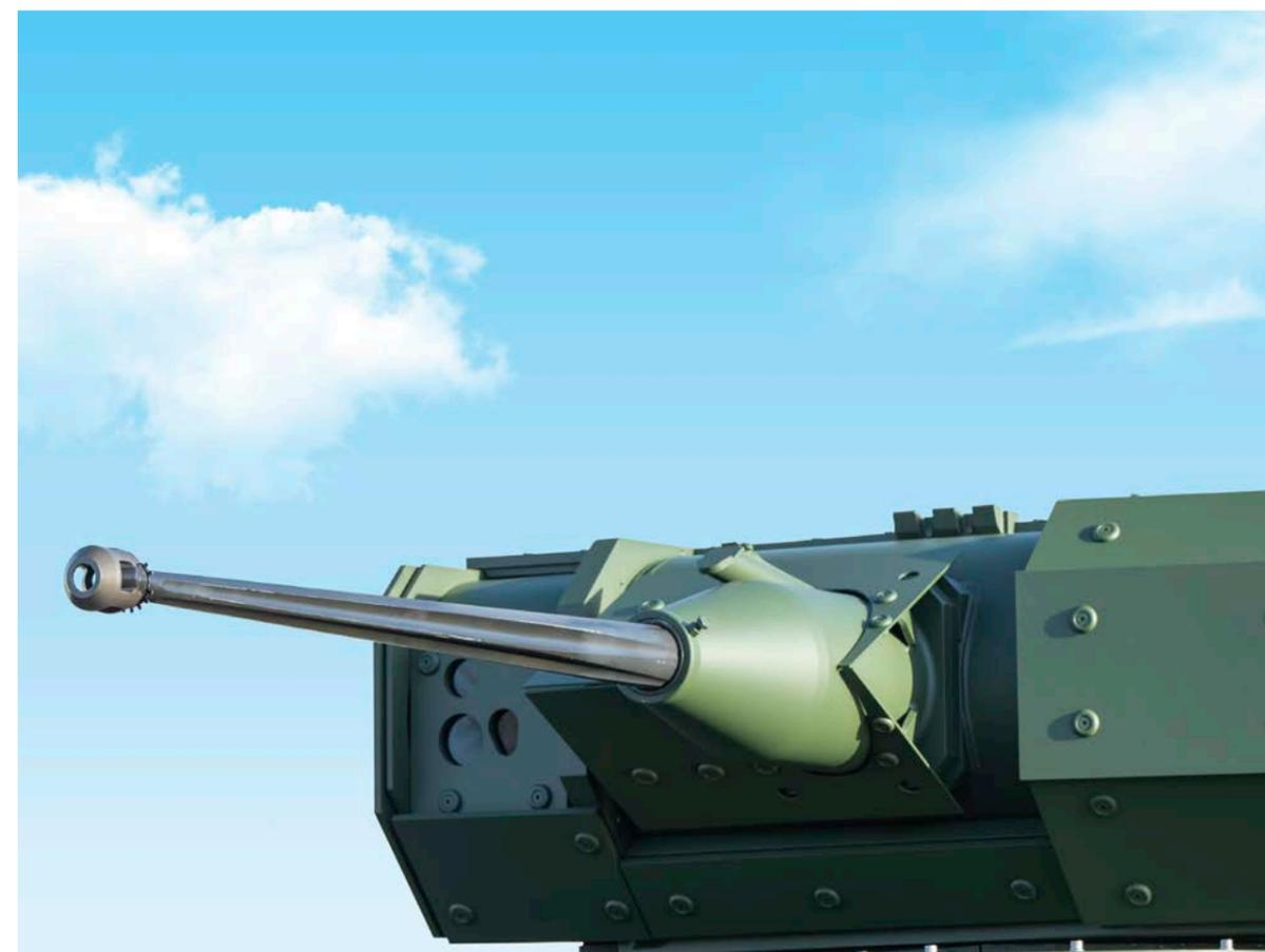
The turret is equipped with an electro-optic sight in order to have effective target acquisition and identification capability on the battlefield. It is also equipped with two-axis independent stabilisation system for fire on the move. The sighting system includes a thermal imager, day sensors and a laser range finder. A commander's 360° panoramic sight can also be integrated if requested by the user.
