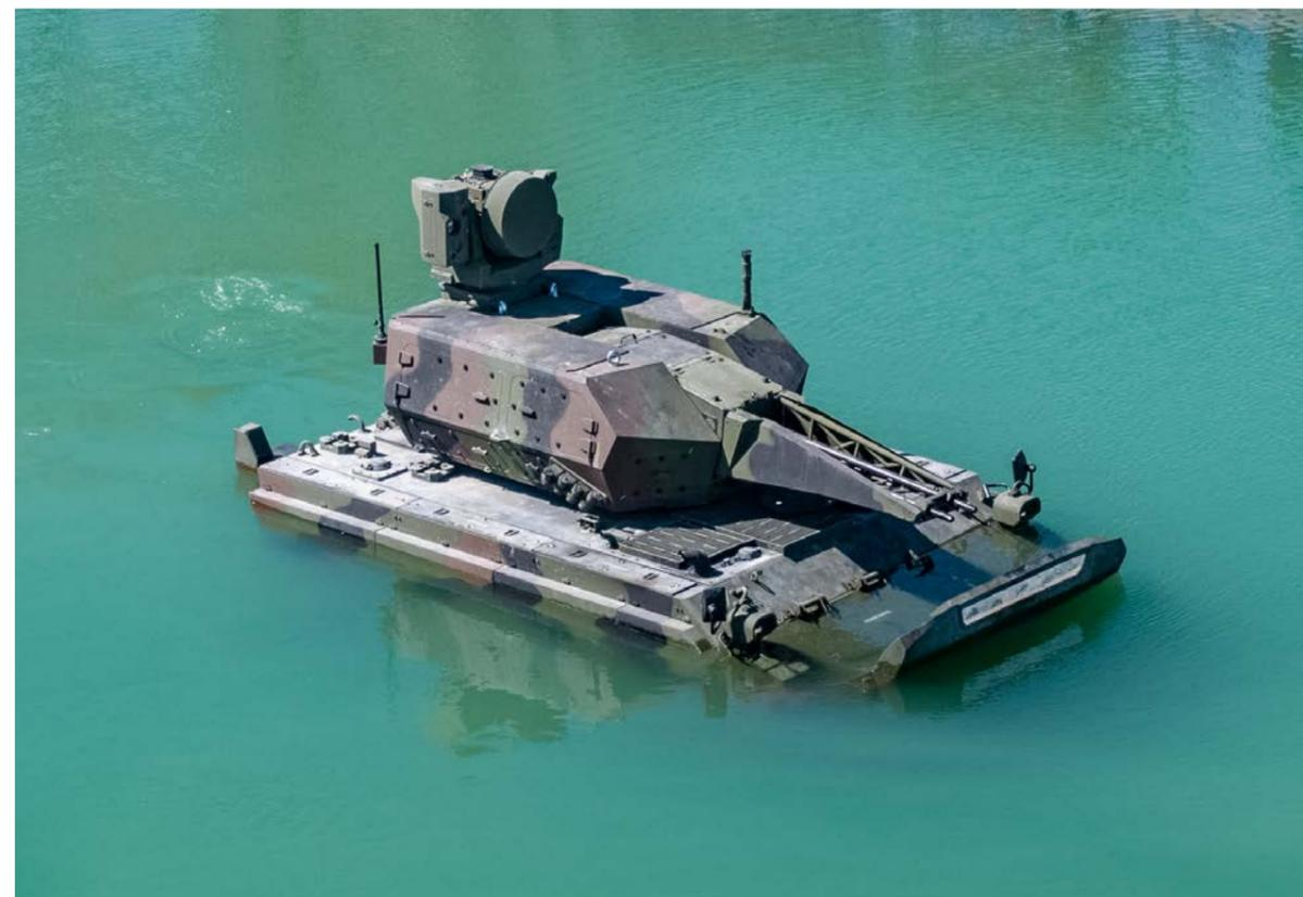
The Command-and-Control configuration designed under the KORKUT Project is fully amphibious and has the capability of propelling itself in deep and/or fast flowing waters.
