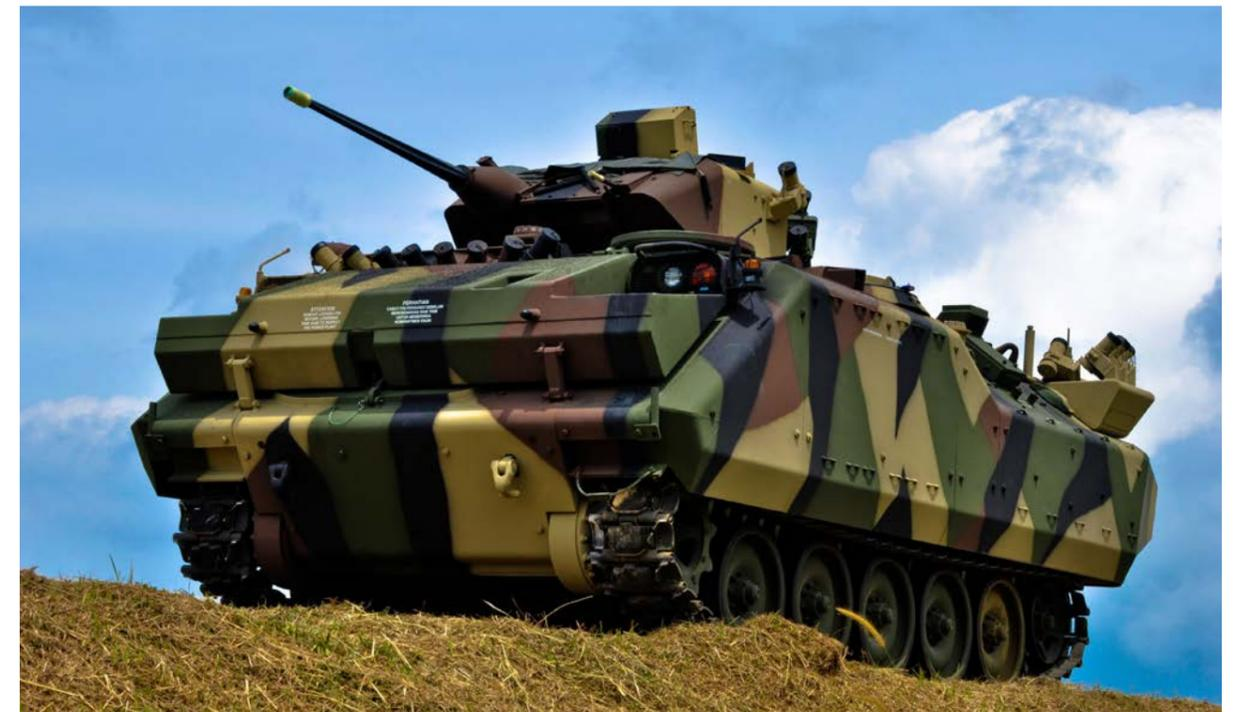
**Armoured Combat Vehicle (ACV) is the generic designation for a tracked, diesel engine powered, heavy armoured platform in the 13-15 tons class, capable of performing combined arms operations with main battle**
