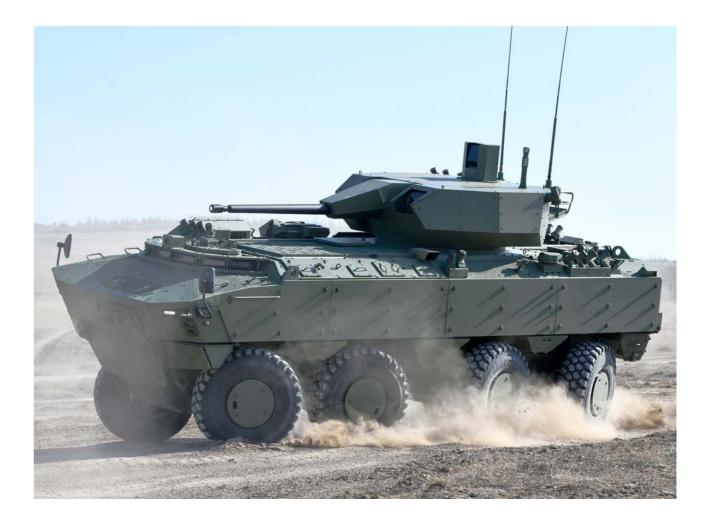
The PARS IV 8x8 superior mobility is due to its power unit, to the balanced load distribution and to the fully independent, height-adjustable, hydropneumatics suspensions designed to support every mission. Thanks to the all-wheel steering system, the vehicle can turn in a radius as long as its length and can easily manoeuvre in urban areas.
