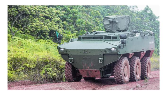
The hull form, underbelly structure, base plates and specially developed mineresistant seats are designed to protect personnel against high-level mine threats. The PARS III 6x6 vehicle runs ahead of its competitors by offering ballistic and mine protections levels similar to MRAP vehicles while maintaining combat and mobility characteristics of modern armoured combat vehicles.
