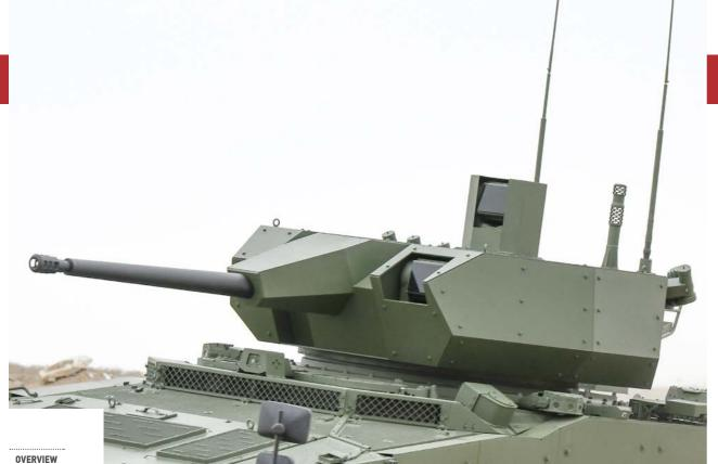
The TEBER-30/35 RCT is a remote controlled turret designed to be installed on wheeled and tracked armoured vehicles and equipped with a medium calibre automatic cannon, an advanced target detection and a fire control system. Unlike conventional turrets, remote controlled turrets do not have any basket structure and thus the extra available interior space provides a significant advantage to the user.
