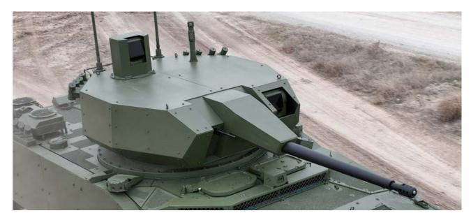
The coaxial MG consists of an electrically operated 7.62 mm chain gun or a gas operated 7.62 mm machine gun. The major advantages of the electrically operated chain gun are that a misfired round can be extracted by the electrical drive and the gun can continue firing without any crew served action, and that the highly toxic propellant gas that occurs after firing is significantly reduced compared to conventional gas operated machine guns.
