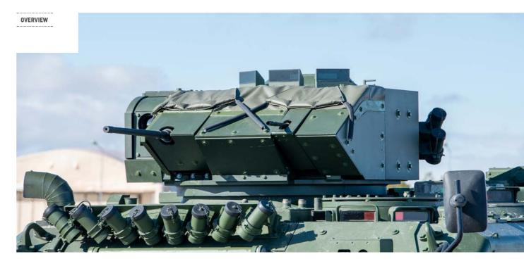
The SABER is a medium calibre oneman, power operated turret that can be fitted on wheeled and tracked armoured vehicles.
