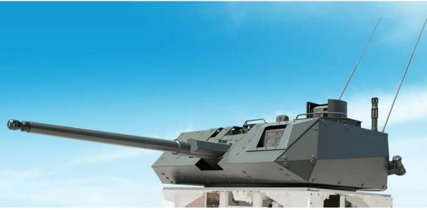
SuperShot 40 mm (40x180 mm) ammunition can also be used in the turret as the 30 mm cannon can be easily converted by a simple replacement on the field to fire those 40 mm rounds.
