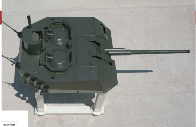
The TEBER-30 Two-Man Turret, is a medium caliber turret that can be fitted to wheeled and tracked armoured vehicles and is offered in two configurations. In the conventional two-man configuration, the commander and the gunner are positioned in the turret basket.
