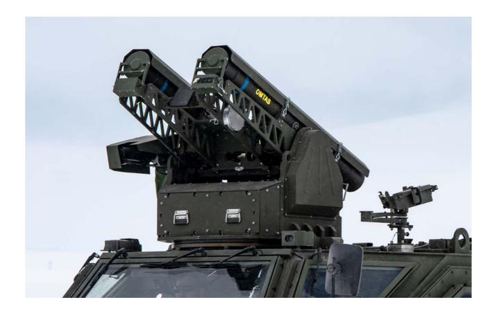
Capable of performing continuous 360 degrees traverse, the ARCT is armed with two anti-tank guided missiles along with a 7.62 mm coaxial machine gun. By means of its digital fire control system, the turret can automatically perform all the necessary ballistic calculations for achieving the highest hit probability, with both the missiles and coaxial machine gun. The gunner's sight system includes
