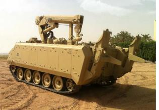
The M113A4 Recovery Vehicle is the next generation modernized version of the M806 vehicle. It is fitted with a hydraulic crane mounted on the vehicle's top plate and a hydraulic recovery winch with a fairlead assembly mounted inside the vehicle, which facilitates the recovery and towing of both armoured and non-armoured vehicles in difficult terrain. It is armed with a self-defence 12.7 mm MG and carries 3 personnel including driver, gunner and technician.
