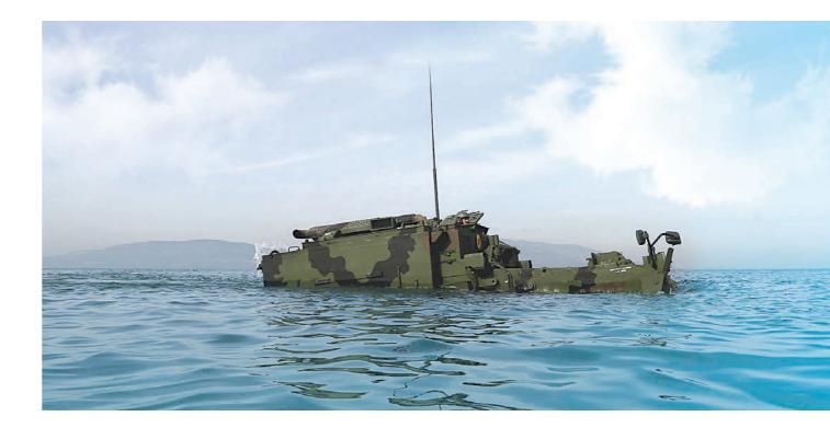
One of the most important and unique features of the AACE is its amphibious capability. It can be operated with a crew of 2. In addition, the AACE is fitted with modern electronic systems such as day and night cameras, multi-function LCD monitor and air-conditioning system.
