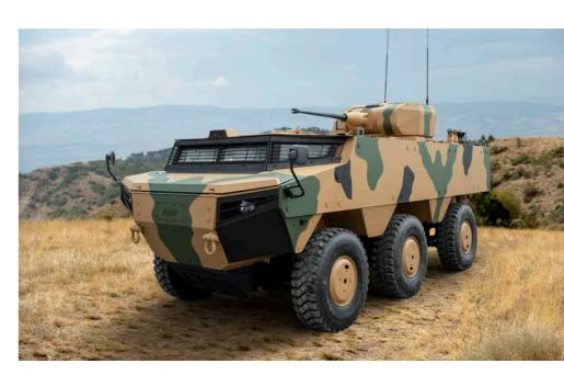
balanced design, the vehicle's axle loads are almost equal. This design approach provides the vehicle with the ability to move comfortably even on loose, soft and rough terrain while also providing maximum control at high-speed and short braking distances. The central tire inflation system (CTIS) allows the driver to adjust tire pressure to suit different terrains, and the hydro-pneumatic suspension system provides the best road holding and ride height for different road conditions.
