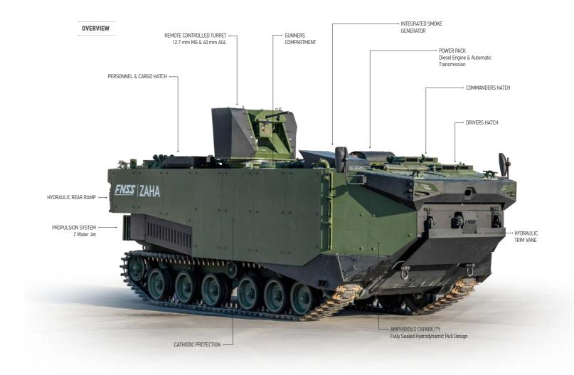
is the latest technology amphibious vehicle designed by FNSS to meet amphibious operational requirements.
