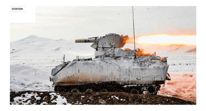
Armoured Combat Vehicle (ACV) is the generic designation for a tracked, diesel engine powered, heavy armoured platform in the 13-15 tons class, capable of performing combined arms operations with main battle tanks. The platform design allows integrating different subsystems for executing a variety of different roles. The Armoured Personnel Carrier (APC) chassis forms the base vehicle for all other members of the ACV-15 Family of Vehicles.
