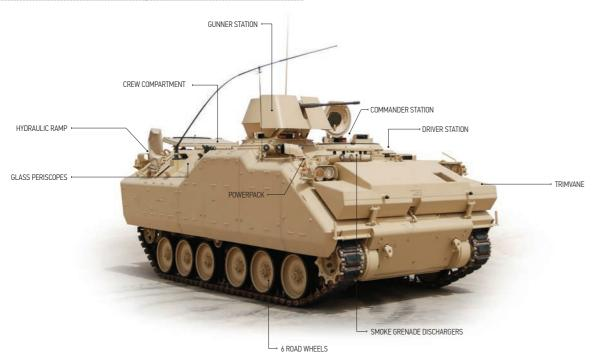
The vehicle is upgradeable thanks to its growth potential and its configuration can be tailored in accordance with user requirements into a true family of vehicles that can be utilized as cavalry, infantry, MBT's support vehicles and artillery.
