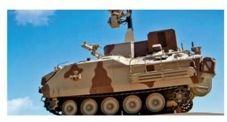
The FITTERS variant is the Recovery & Maintenance Vehicle configuration of the ACV-15 FoV. It is distinguished by the large hatch on top of the hull and the hydraulic crane capable of lifting a complete powerpack if required. The additional flotation panel on the trim vane helps compensate for the weight of the hydraulic crane. It is armed with a self-defence 12.7 mm MG and can carry 4 personnel including driver, gunner and two technicians.
