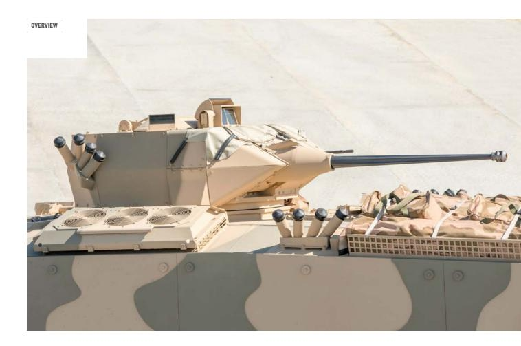
The SABER is a medium calibre one-man, power operated turret that can be fitted on wheeled and tracked armoured vehicles.
