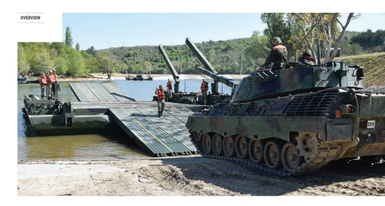
The OTTER is a bridge and ferry system designed for safe and fast transport of combat and logistic military vehicles in river crossing operations.
