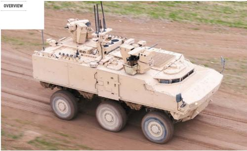
The turrets are fitted with a universal weapon mount which enables them to carry 7.62 mm, or 12.7 mm machine guns, or 40 mm automatic grenade launchers, which can be easily changed depending on mission requirements. Two-axis stabilisation allows firing on the move and the high maximum elevation of the guns enables to engage targets on high grounds (building tops, cliffs etc) and/or low altitude aerial targets.
