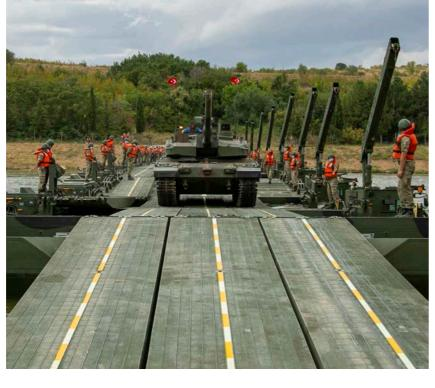
In terms of self-sufficiency, the OTTER can carry four ramps on a single system, which eliminates the need for additional logistic vehicles. The OTTER is also fitted with a self-recovery winch, which recovers the vehicle or any other system especially in soft terrains.
