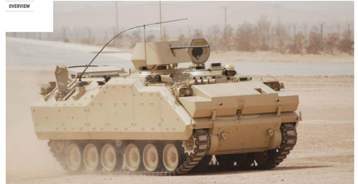
**The ACV-19 (Armoured Combat Vehicle) is the general name for 15-19 ton weight class, modern high performance vehicles derived from the highly successful FNSS ACV. These vehicles have proven themselves with numerous armies worldwide. The ACV-19 offers the latest developments in high value vehicle performance for internal volume and payload but maintains the advantages of commonality with the ACV family of vehicles.**
