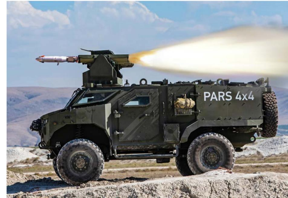
The mobility of the PARS 4x4 is enhanced by its central tire inflation system, and it also has a run flat capability thanks to its in-tire solid disc system. The PARS 4x4 can reach a maximum speed of 110 km/h on road and has a range of 700 km. It is fitted with an automatic transmission with an axle lock to enhance mobility on slippery surfaces and soft soil.
