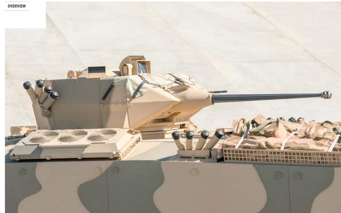
**The SABER is a medium calibre one-man, power operated turret that can be fitted on wheeled and tracked armoured vehicles.**
