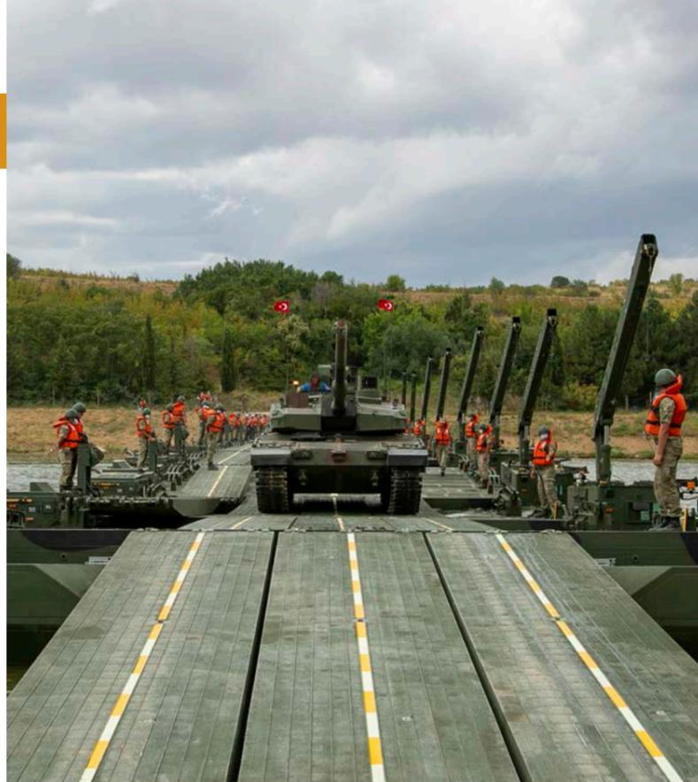
In terms of self-sufficiency, the OTTER can carry four ramps on a single system, which eliminates the need for additional logistic vehicles. The OTTER is also fitted with a self-recovery winch, which recovers the vehicle or any other system especially in soft terrains.
