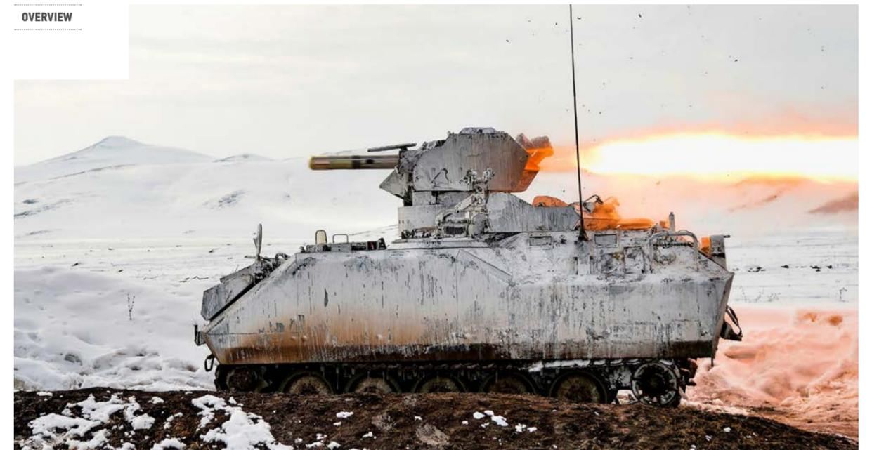
**Armoured Combat Vehicle (ACV) is the generic designation for a tracked, diesel engine powered, heavy armoured platform in the 13-15 tons class, capable of performing combined arms operations with main battle tanks. The platform design allows integrating different subsystems for executing a variety of different roles. The Armoured Personnel Carrier (APC) chassis forms the base vehicle for all other members of the ACV-15 Family of Vehicles.**
