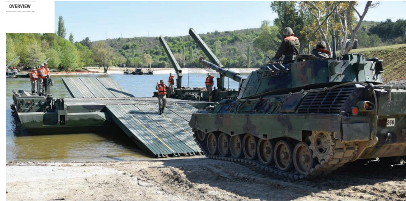
The OTTER is a bridge and ferry system designed for safe and fast transport of combat and logistic military vehicles in river crossing operations.
