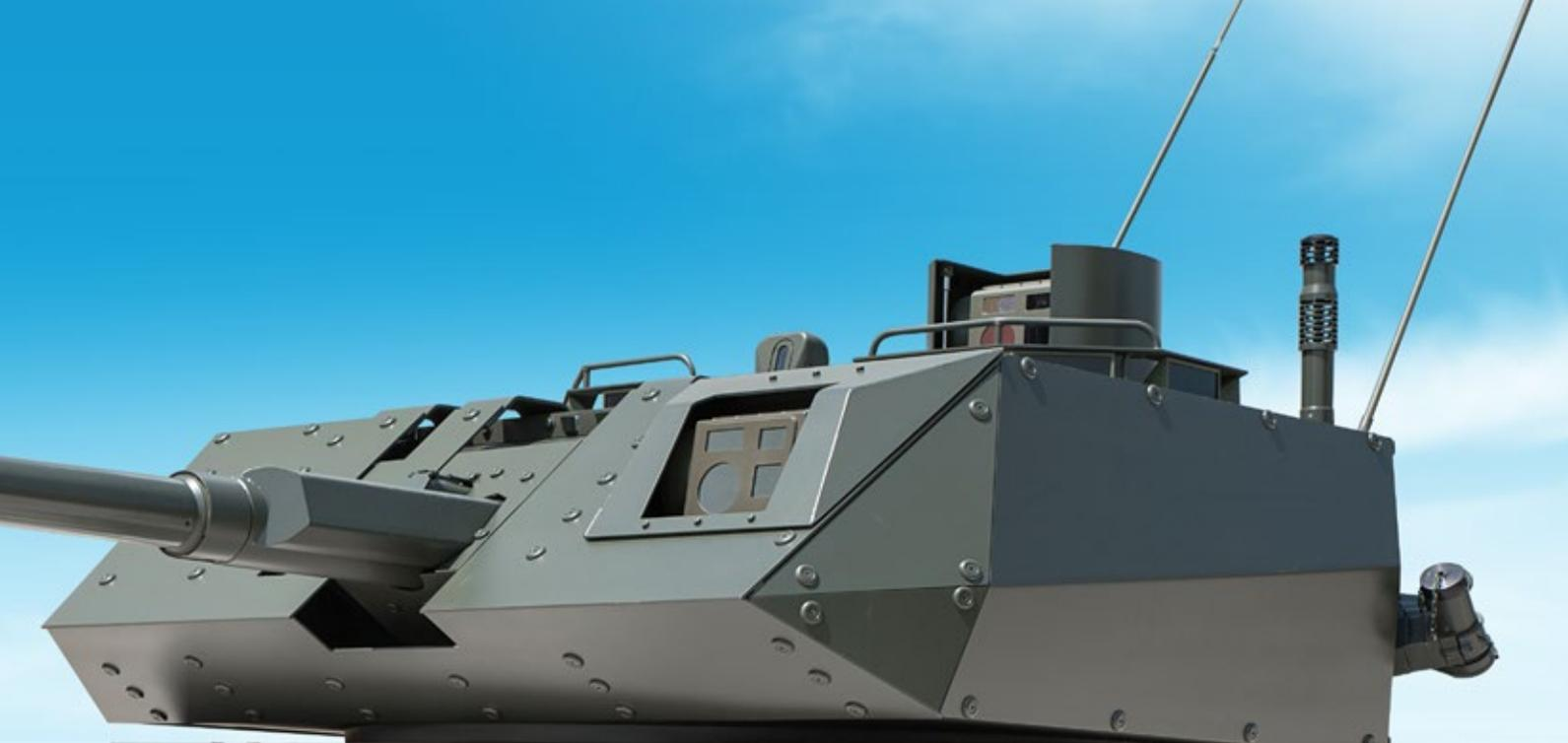
***SuperShot 40mm (40x180mm) ammunition can also be used in the TEBER-30 Two-Man Turret. The 30mm canon can be easily converted by a simple replacement on the field to fire SuperShot 40mm ammunition.***
