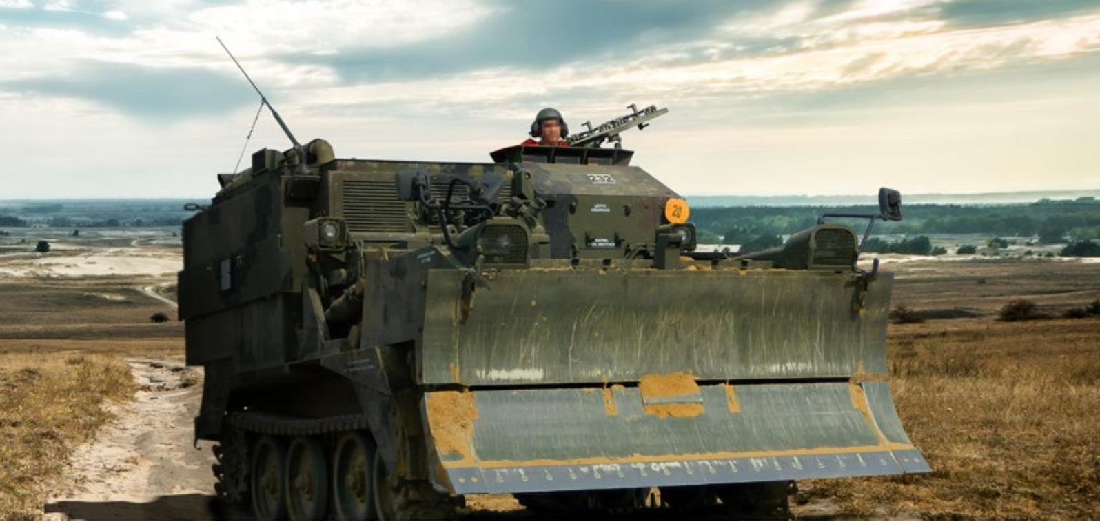
AACE' power pack consists of fully automatic transmission, coupled with a diesel engine. AACE is capable to speed up to 45km/h on land. It can travel safely in river streams against current speeds up to 1.5 m/sec with 360° high-maneuverability through its two water jets, placed at the rear section on both sides of the vehicle.
